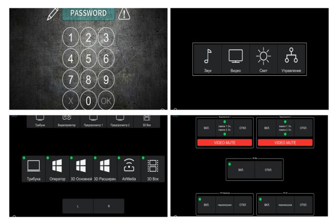
In the multimedia system it is possible to switch audio and video from any source of the system to any means of displaying the system, whether it is an interactive podium (USB-Flash drive or connected tablet/laptop), operator's PC, document camera or even a laptop or any other mobile device in the room, connected to the system via wifi.
